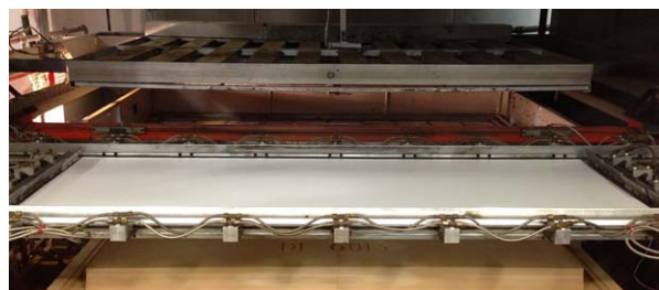
Figure 7. Experimental setup of 36x73 in. HIPS sheet pinned all the way around (sample A of Table 4).
